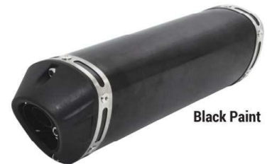
TR041A-BK S/Steel 304 / Aluminum Material ABS / With DB Killer Body Length = 300mm Inlet Diameter = 38mm Body Diameter = 100 x 90mm
