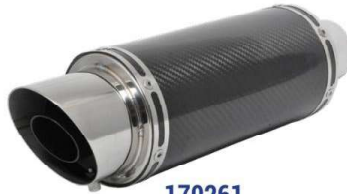
170261 S/Steel 304 / Carbon "Rossi" style Body Length = 250mm Inlet Diameter = 60mm Body Diameter = 115mm With DB Killer TD=89mm
