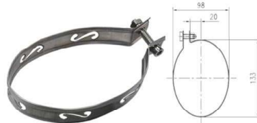
TR1001-OC Stainless Steel Clamp Body Diameter = 133x98mm Off Center
